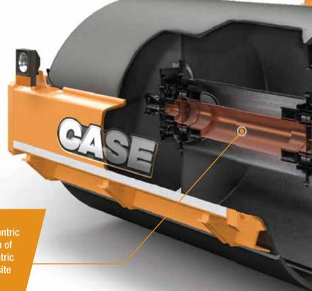
The centrifugal force is generated by an internal eccentric shaft and a rotating mass: depending on the direction of rotation, the rotating mass is in phase with the eccentric shaft for a maximum centrifugal force or in the opposite position, for a minimum centrifugal force.
